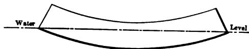
Fig. 1436.—After the preceding experiment the same bar was reheated and reversed in the water, the eleventh cooling resulting in the above form, the bar bending in the opposite direction from that previously shown.
