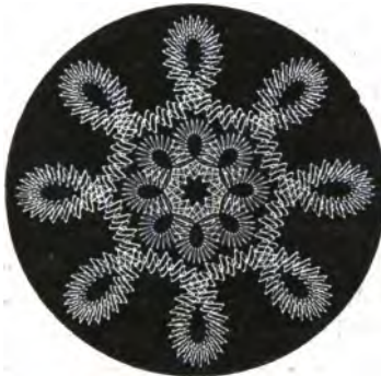
Geometric Chuck combined with the Rose Engine.
