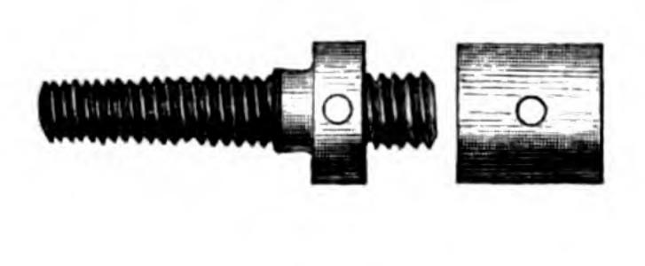
19, are of metal: A is the male, B the female chuck. The male chuck is made to screw on the mandril end. The projection in front is cut with a fine screw thread, such as is used for the covers of fancy boxes. The
