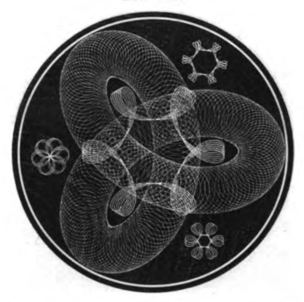
were cut in the lathe by its aid, and are the result of three circular movements in the same plane. These illustrations will, however, give but a small idea of the immense variety of figures the compound geometric chuck will execute.
