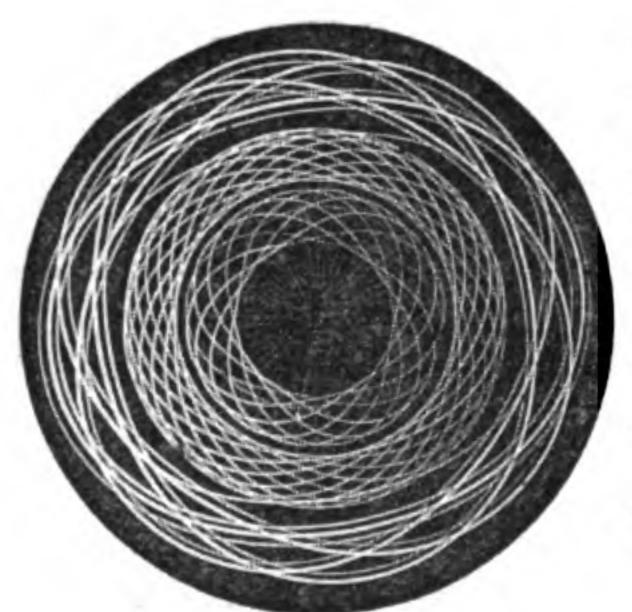
the division wheel of the chuck, on setting the lathe in motion, and applying the tool between each movement, a series of ellipses will be arranged equally around the central point of the wood, and the figures produced will be like those at Fig. 192.
