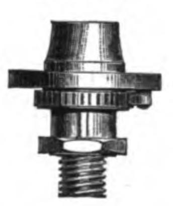
The chuck itself forms part of a set of apparatus for spiral turning. Through the medium of this contrivance the lathe-spindle is connected with the slide-rest screw by change-wheels, which act in precisely the same manner as in the self-acting lathe already described.
