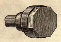
thickness, say one inch, and saws the corners off, so that it is eight-sided. It is then ready to screw on the face plate of the lathe. This is quickly done by having small screw holes in the plate for this purpose, as shown in Fig. 1, page 17.
