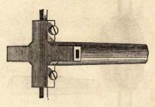
37. It is merely a cross, formed on the end of a center fitting the back spindle, the same as the lathe center does. The arms of the cross are made stout and thick, so as to admit of a square hole being cut in them. The hole is made by
