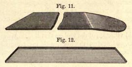
There is no occasion to make the ends at different angles, except the convenience, before stated, of having four cutting edges on one piece, for any angle can be easily given by the position of the hand or the direction of the rest. These tools, here alluded to, are only to be used when the job has been all turned true and the scale removed; they *scrape*, merely, they do not cut.
