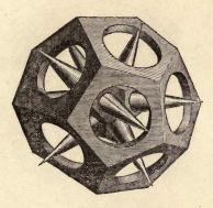
spurs turned inside. At first sight it would appear that the tool, severing the rings, would cut off the points also, but it will be seen that this is not the case, for the holes being bored so as to
