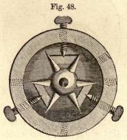
Fig. 48 shows how the points are turned. After the internal rings are cut out with a quadrant tool like Fig. 49, and the spur also severed, by cutting in the ends of the holes (not boring them out solid), the globe is put in a shell chuck, with three set screws in it, as shown. The set screws go through the holes in the globe, and the cross
