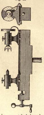
whole should be accurately balanced, or else the work will be full of chatters or ridges. Since centrifugal force increases as the square of the velocity, any thing that runs a little out of truth, will be very much exaggerated as the speed increases. By using cutters of different shapes, beautiful effects can be produced; as, for instance, suppose we take a common round-nose cutter, set the index so as to divide the circle of the job we are to work on in twenty-four parts, and execute
