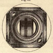
ball, left inside the exterior shell. One side of it is squared up before the ball is cut free from the globe, and the job is then reversed and the other side squared. The ball is then cut free, and the
