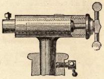
This is simply a casting fitted with a screw and spindle, as shown. The spindle has a tool let in the front end and held there by a set screw, and there is a wheel at the back end to run the spindle in and out. The casting has a leg to it which
