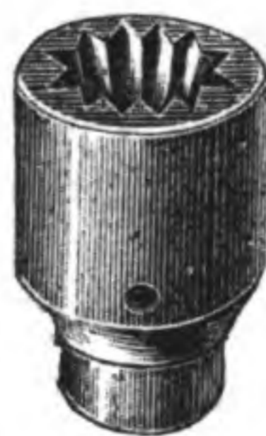
FIG. 7.—SELF-CENTREING CHUCK (WOOD).
