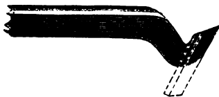
FIG. 17.—PRINCIPLE OF LOOSE CUTTERS.
