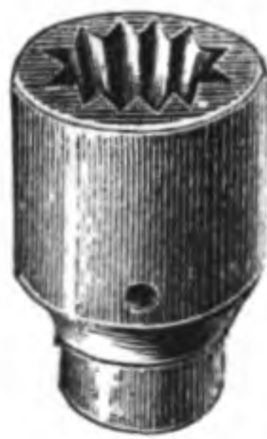
FIG. 7.—SELF-CENTREING CHUCK (WOOD).
