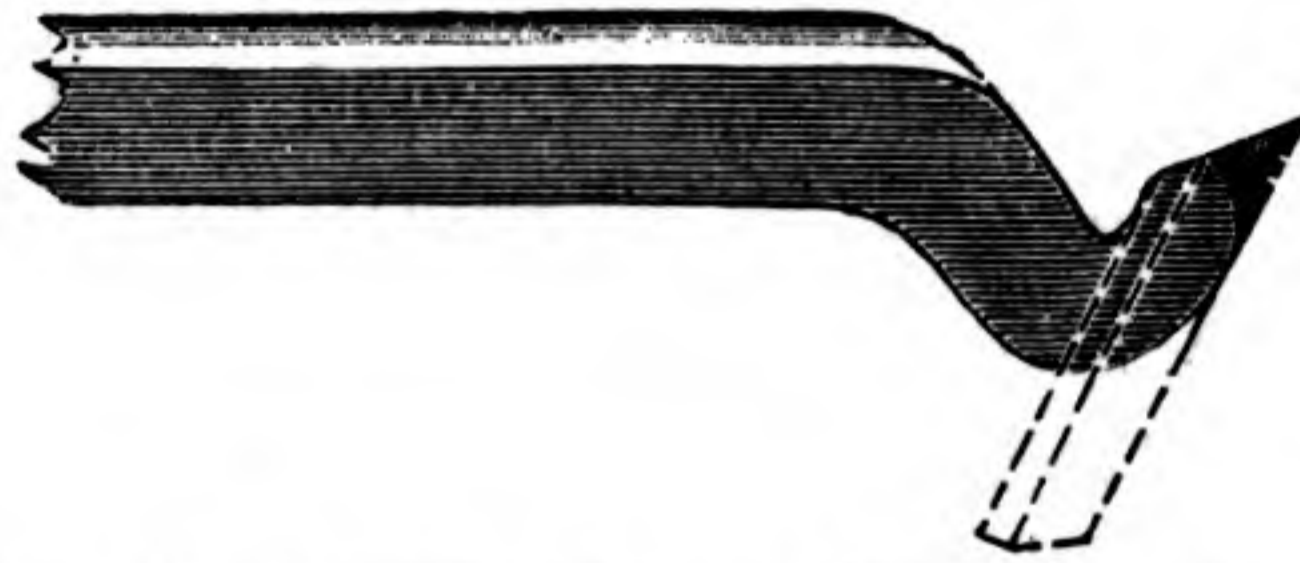
FIG. 17.—PRINCIPLE OF LOOSE CUTTERS.
