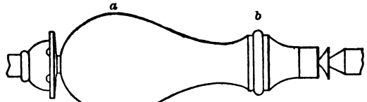
FIG. 4.—BRADAWL HANDLE: FINISHED.
