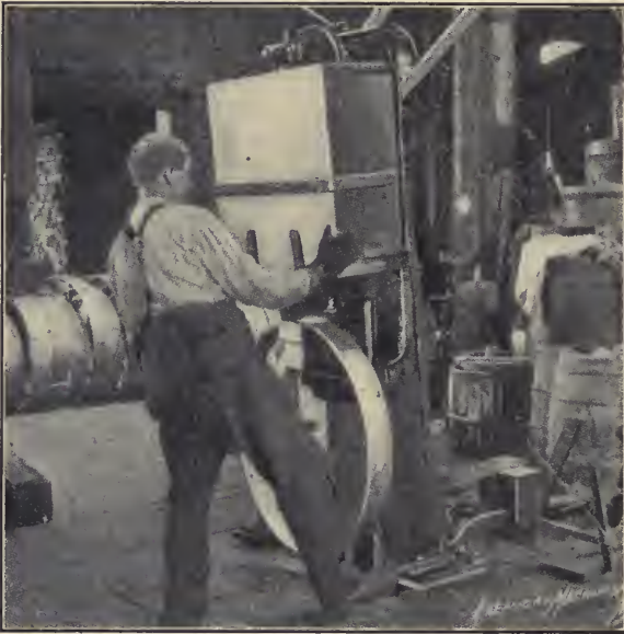
FIG. 201.—Welding wagon-wheel rims on Justice hammer.
