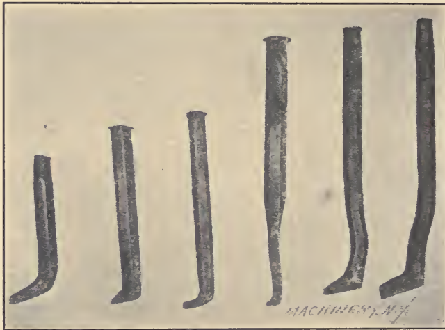
FIG. 12.—Staking-tools used for repairing dies.
