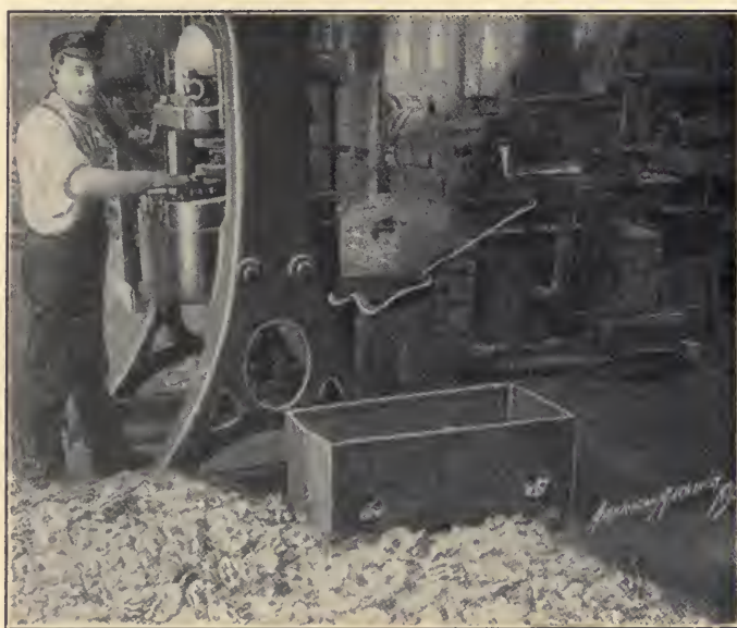
FIG. 206.—Wheel-flange, muffle and forming-press.
