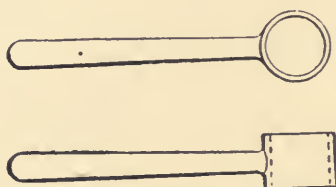
FIG. 28.—Drop-forged shell and handle for ratchet drill.
