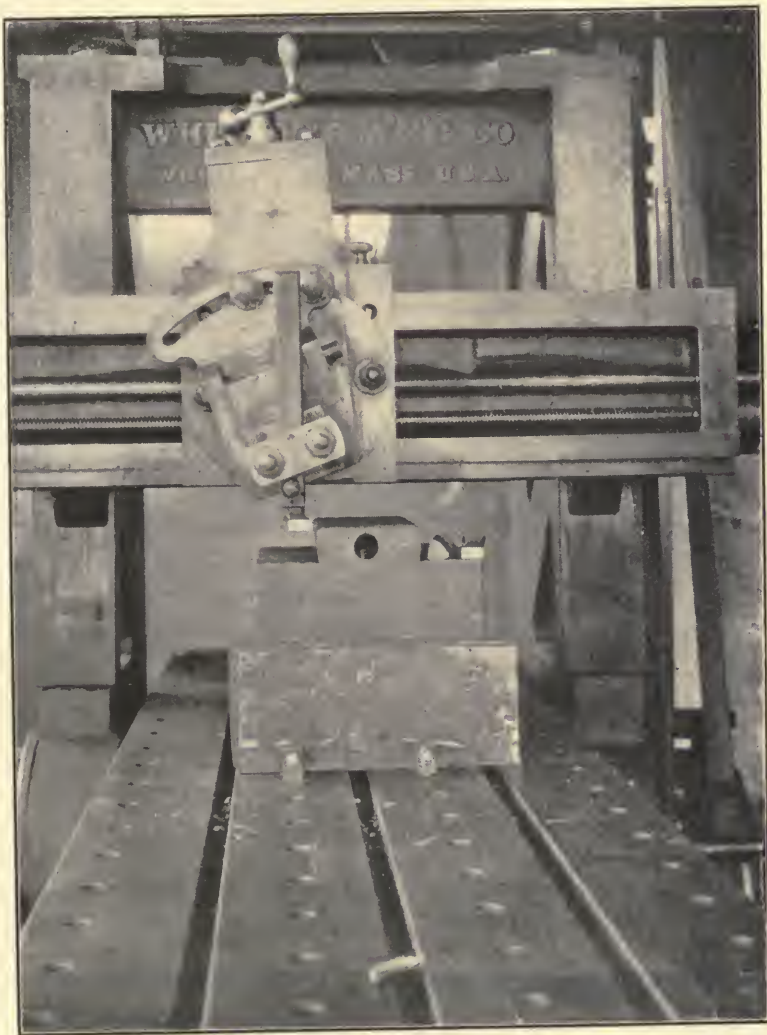
FIG. 297.—Shanking dies with high-speed cutting tool.
