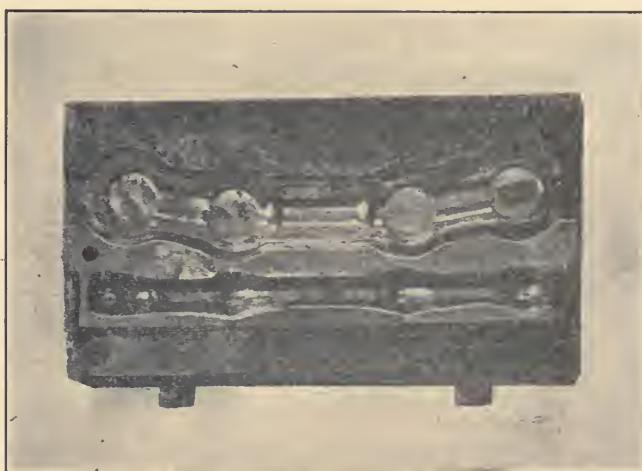
FIG. 15.—Drop-forging die, showing bending-form in front.
