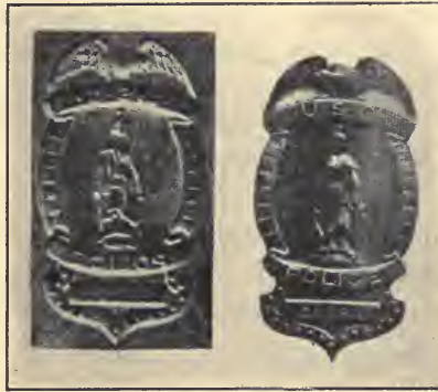
FIG. 79.—Embossed Police-shield before and after trimming.
