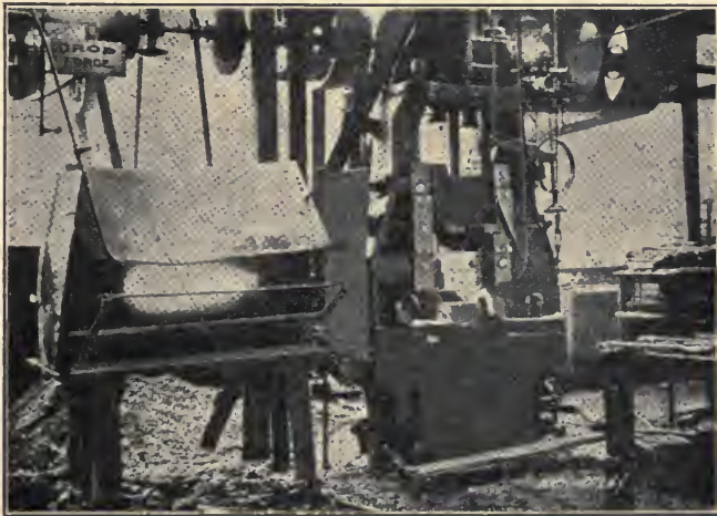
FIG. 20.—Oil-heating furnaces and drop-hammer.
