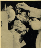
Grinding a Spiral Flute Cutter on 375-2 Cutter Grinder with 717-1 Universal Tool Head
