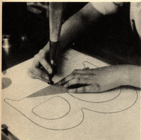
When a letter design has been approved, it goes to a specially designed machine of great accuracy to be reproduced as the large brass letter which is to serve as master pattern for making the punch. The picture shows the operation.
