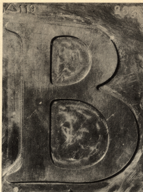
The brass letter, or letter pattern, actual size. The surrounding metal has all been routed away, leaving the letter high and sharp in relief. These brass letters are the master patterns for Linotype faces.
