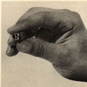
The finished punch. When a punch has passed the system of microscopic inspections and other tests and examinations, it is hardened in an electric furnace, finished by grinding and lapping, and again reinspected and retested.
