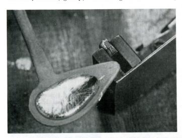
the stick is opened once again and the matrix and the newlycast type are removed (figure 5.) A gentle pressure is all
