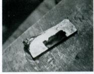
3.) The matrix, now an L-shaped piece of lead, has an exact intaglio replica of the face of the type at one end.
