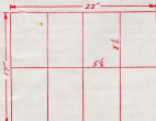
HOW TO CUT SIZE 5\frac{1}{2} \times 8\frac{1}{2} OUT OF A SHEET OF PAPER SIZE 17 \times 22 "
