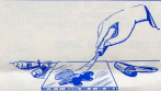
An ink blend on a piece of brass rule and a piece of window glass are desirable, since you can mix ink on the back of a steel palette.
