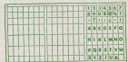
Triple Cap Case. 1 1/2 x 2 1/2 inches will hold three-cap fonts (including points and figures)
