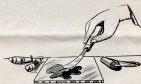
An ink knife or a piece of brass rule and a piece of window glass are desirable, also you can mix tints on the back of a steel plate.
