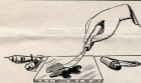
An ink knife or a piece of brass rule and a piece of window glass are desirable, altho you can use inks on the back of a steel galley.
