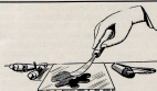
An ink knife or a piece of brass rule and a piece of window glass are desirable, altho you can mix inks on the back of a steel galley.
