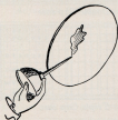
Squirting Oil from Oil Can on Ink Plate to Mix with Ink and Make Cleaning Easier
