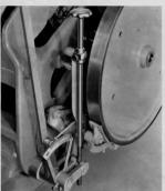
$Figure \ 3-Upper \ Hand \ Wheel \ controlling \\ the \ impression$
