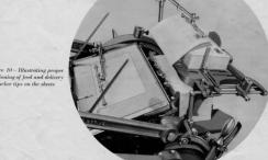
Figure 10 – Illustrating proper positioning of feed and delivery sucker tips on the sheets
