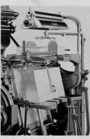
Figure 17—Electric Sheet Dryer in position; a gas sheet dryer or portable spray equipment may also be used
