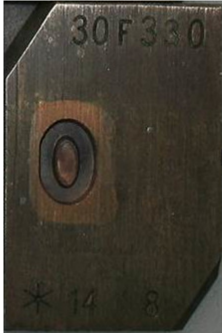
Figure 21: Lanston Display Matrix Marked as Lining Figure
