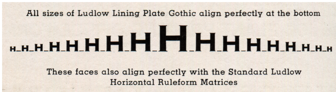
Figure 33: Ludlow Vertical Alignment for Lining Faces
