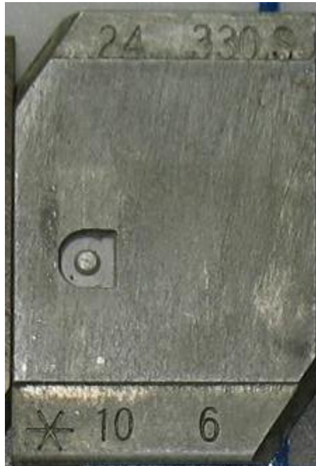
Figure 24: Lanston Series 330, 'S' suffix for alternate character
