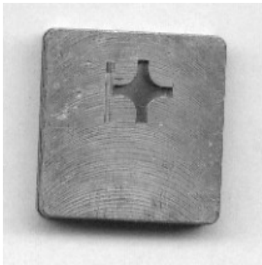
Illustration 5 - English Monotype Mats are 1"x1" and use a cross, as shown for lines standard.
