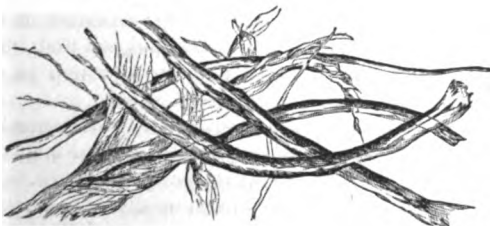
Fig. 3. New official Prussian hemp paper, some cells nearly entire, a few frayed. Magnified 120 times.
