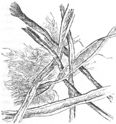
Fig. 1. Fibres from a fine, unsized printing-paper. The flat cells are those of cotton; the rounder ones, of flax; the finer mass below, the entirely frayed remains of both. Magnified 200 times.
