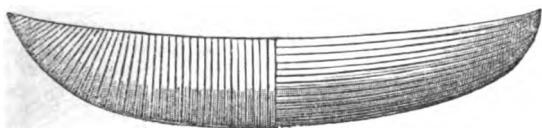
(The alternate fore and aft and cross planking.)
