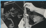
(3) A simple turn of the thumbscrew on the matrix stick holds each line firmly for the Ludlow casting operation. Self-centering and self-quidding sticks offer even greater economies in typesetting.
