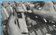
(1) The Ludlow operator gathers a group of matrices from the case and assembles them in a matrix stick proofreading the line at the same time.
