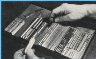
(4) Ludlow all-slug make-up is simple and easy. There is no type to pi, and corrections are quickly and easily made.
