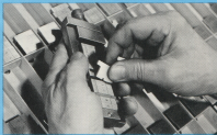
(2) Words and letterspacing is quick and easy. Justification is visible before casting. The spacing units have ears that extend beyond the other matrices making them easy to handle and redistribute.
