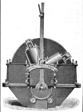
The cut-off is regulated by piston valves which are worked by means of the two spur pinions in connection with a toothed segment and reversing lever. The engine is com-pletely covered in, but the top cover has been removed to show some of the cylinders and the attachment of the piston rods to the flywheel disk. The engine indicates 13 h.p., with 80 lb. boiler pressure, and at § cut-off. The cylinders are 6 in. diam. by 3 in. stroke, and the maximum speed is 450 revolutions er minute.
