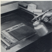
The entire form is sprayed with an opaque solution which dries upon contact with form.
