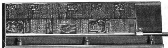
THIS CUT SHOWS THE LOCK HOLDING TWO COLUMNS OF MATTER.
