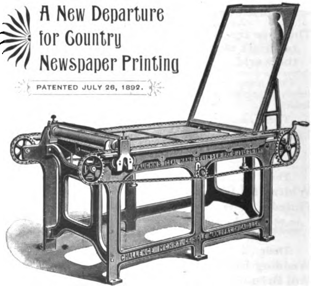
ILLUSTRATION SHOWING IDEAL PRESS READY FOR LOWERING TYMPAN AND TAKING IMPRESSION.
