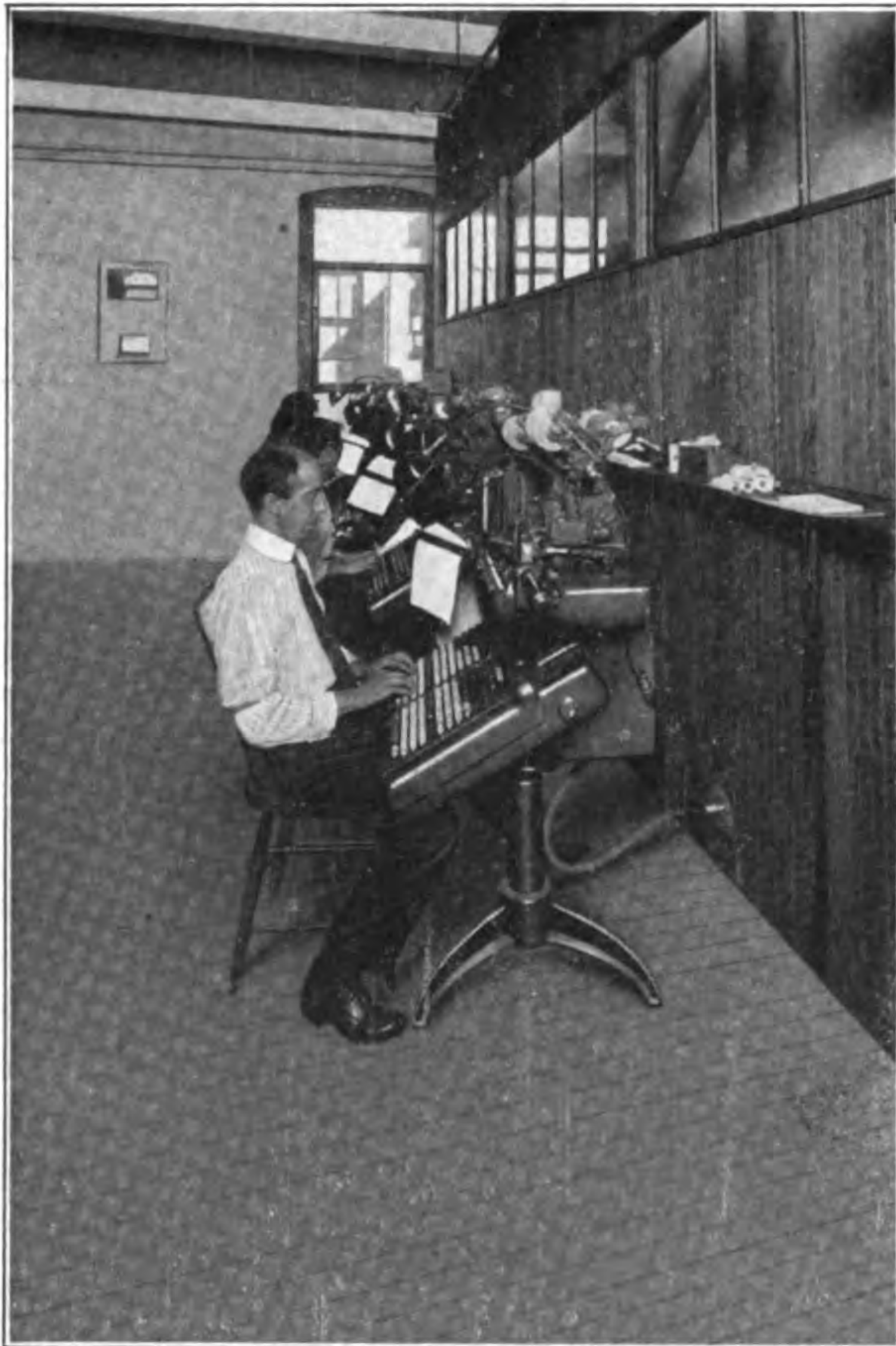
These four Monotype Keyboards and five Casting Machines at the Atlantic Printing Company furnish all the composition as well as type and rule used on the Boot and Shoe Recorder , and twenty-three other publications, as well as catalog and job work. A complete Non-Distribution System makes the work of the hand compositor easy in the composing room
