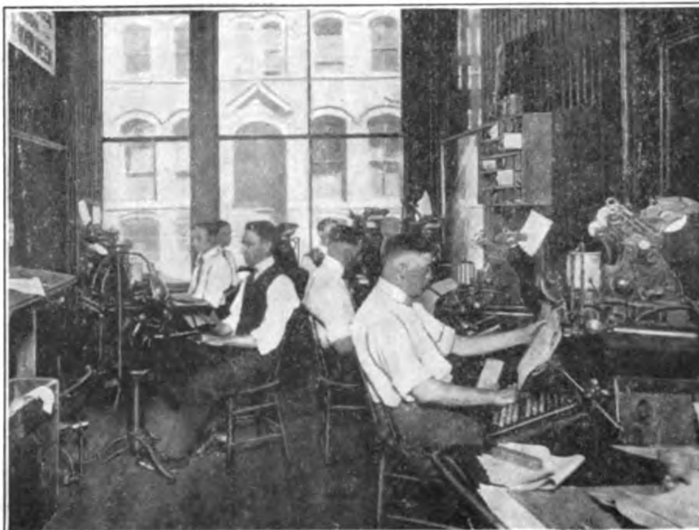
Six Monotype Keyboards take care of all composition on the Telegram —news matter as well as ads
