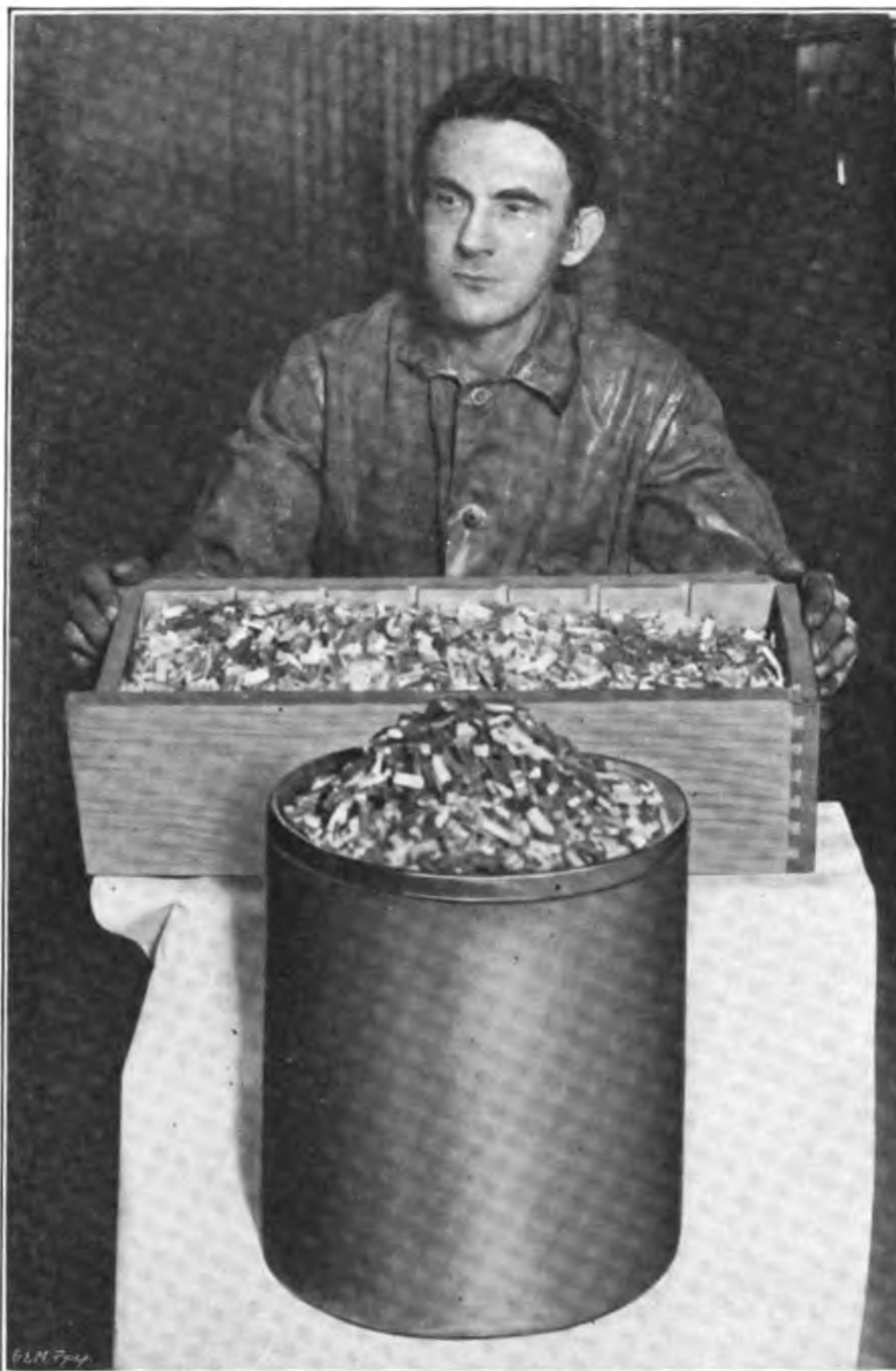
The box and the can hold 274 pounds of Monotype quads cast in five hours
