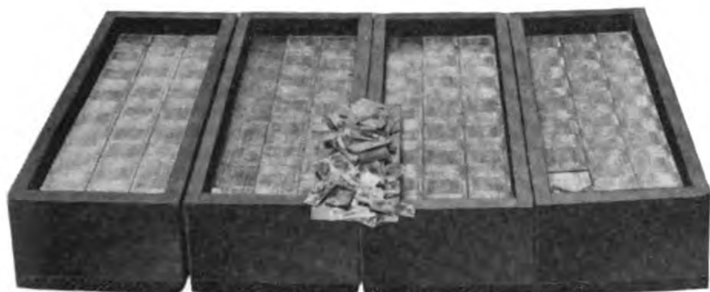
Four hundred and thirty-two pounds of 2 point, 12½ pica single column leads, cast in seven hours
