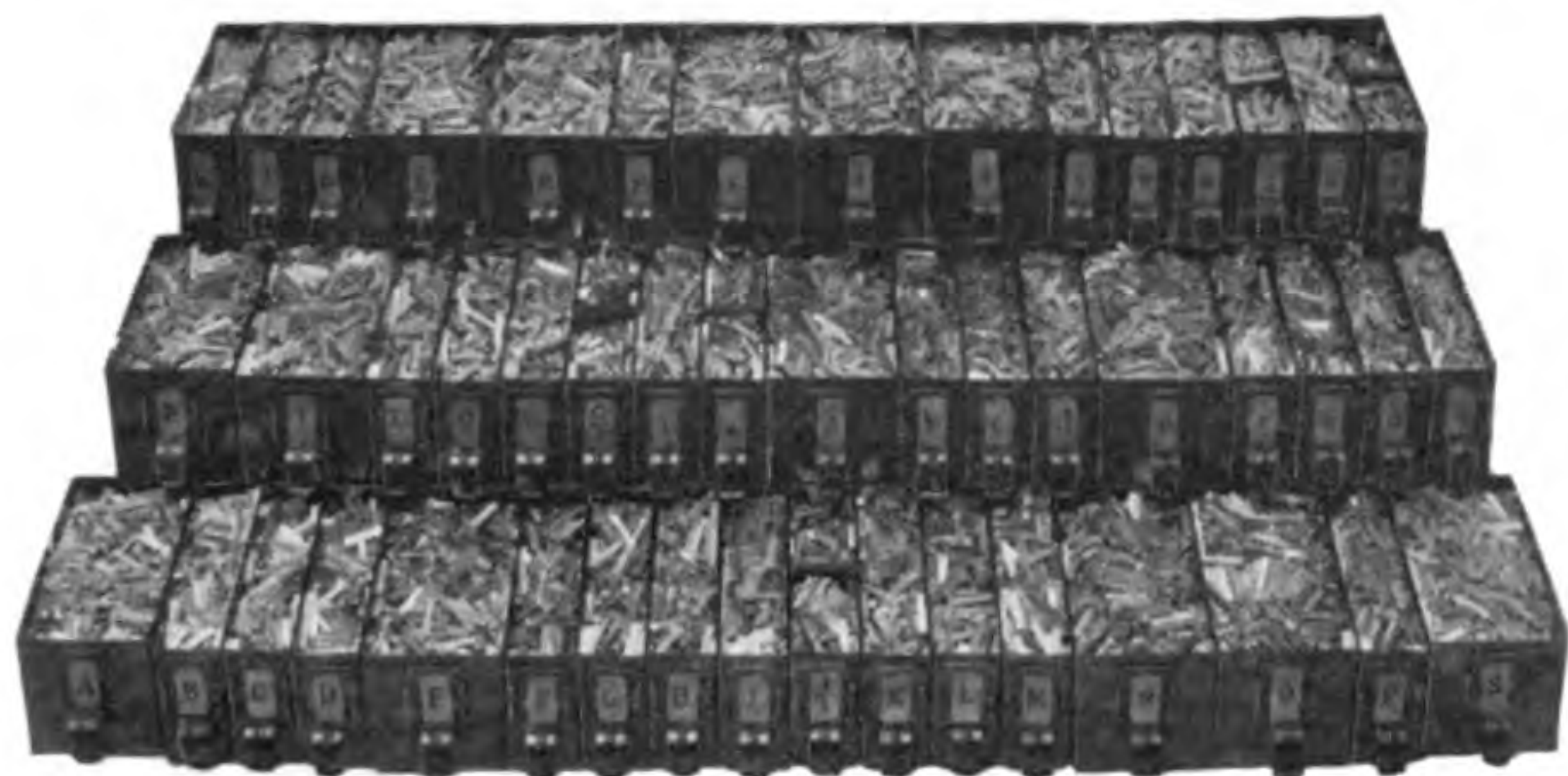
One hundred and sixty-five pounds of 12 point No. 118J, cast in six hours
