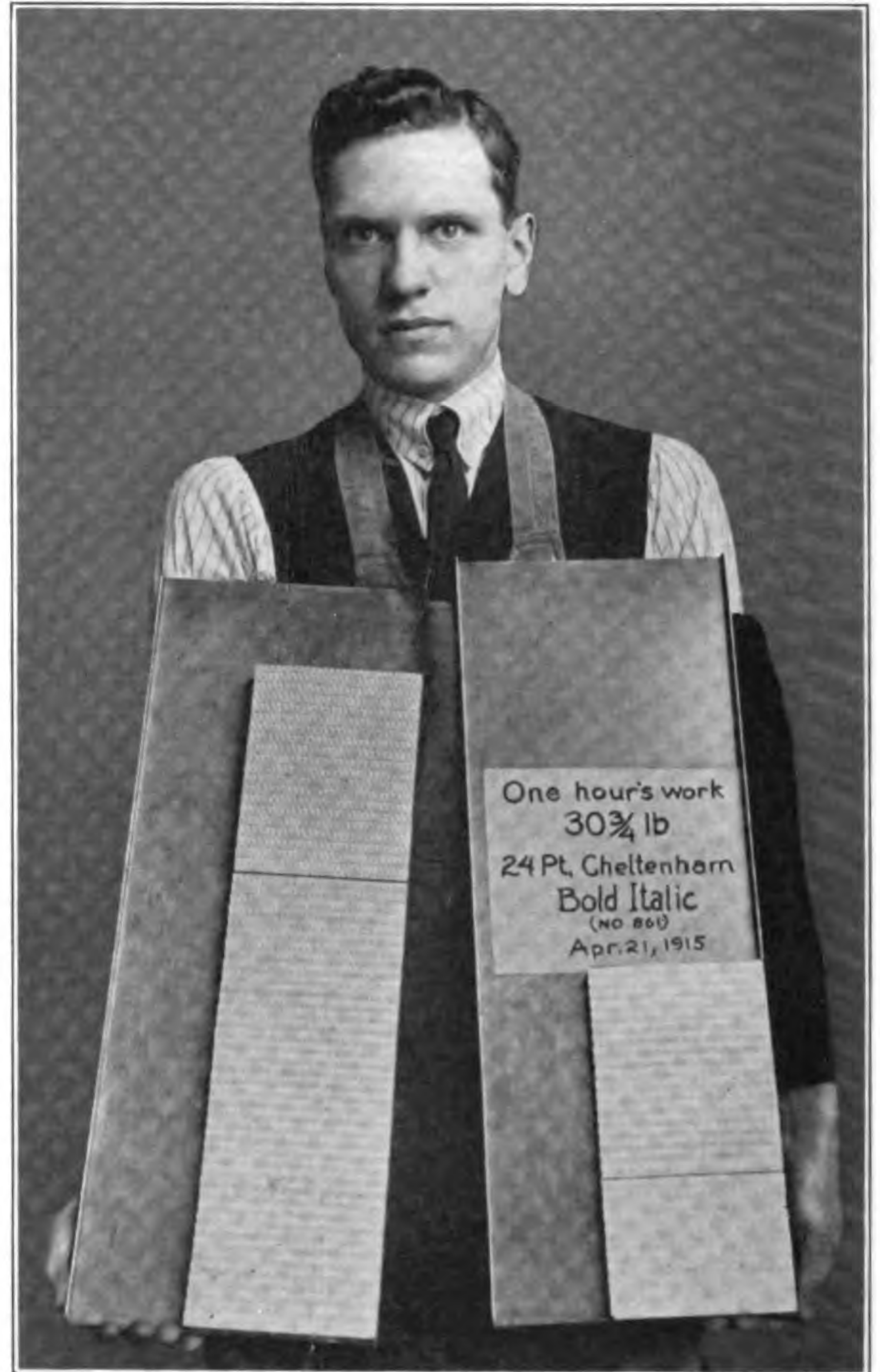
The galleys show one hour's product from the Monotype at the National Cash Register Co., Dayton, Ohio.
