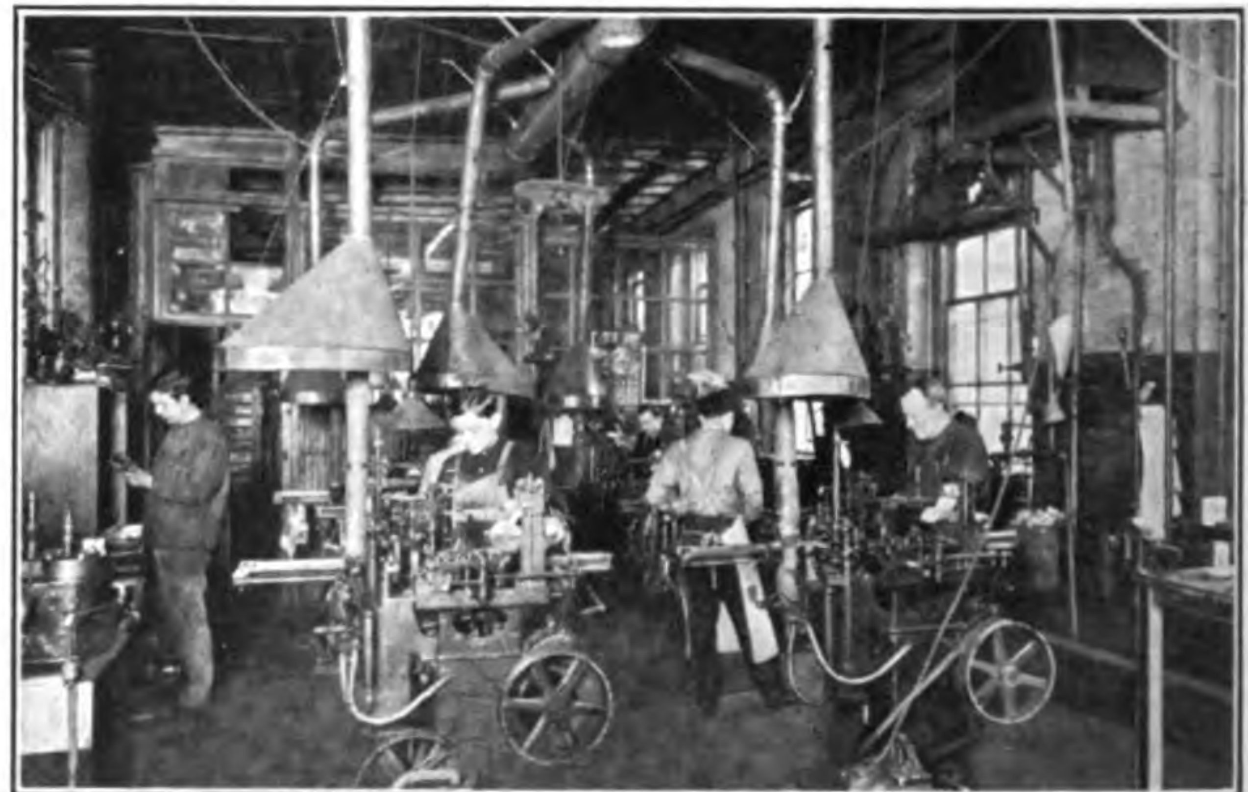
Monotype Casting Machines in Operation
