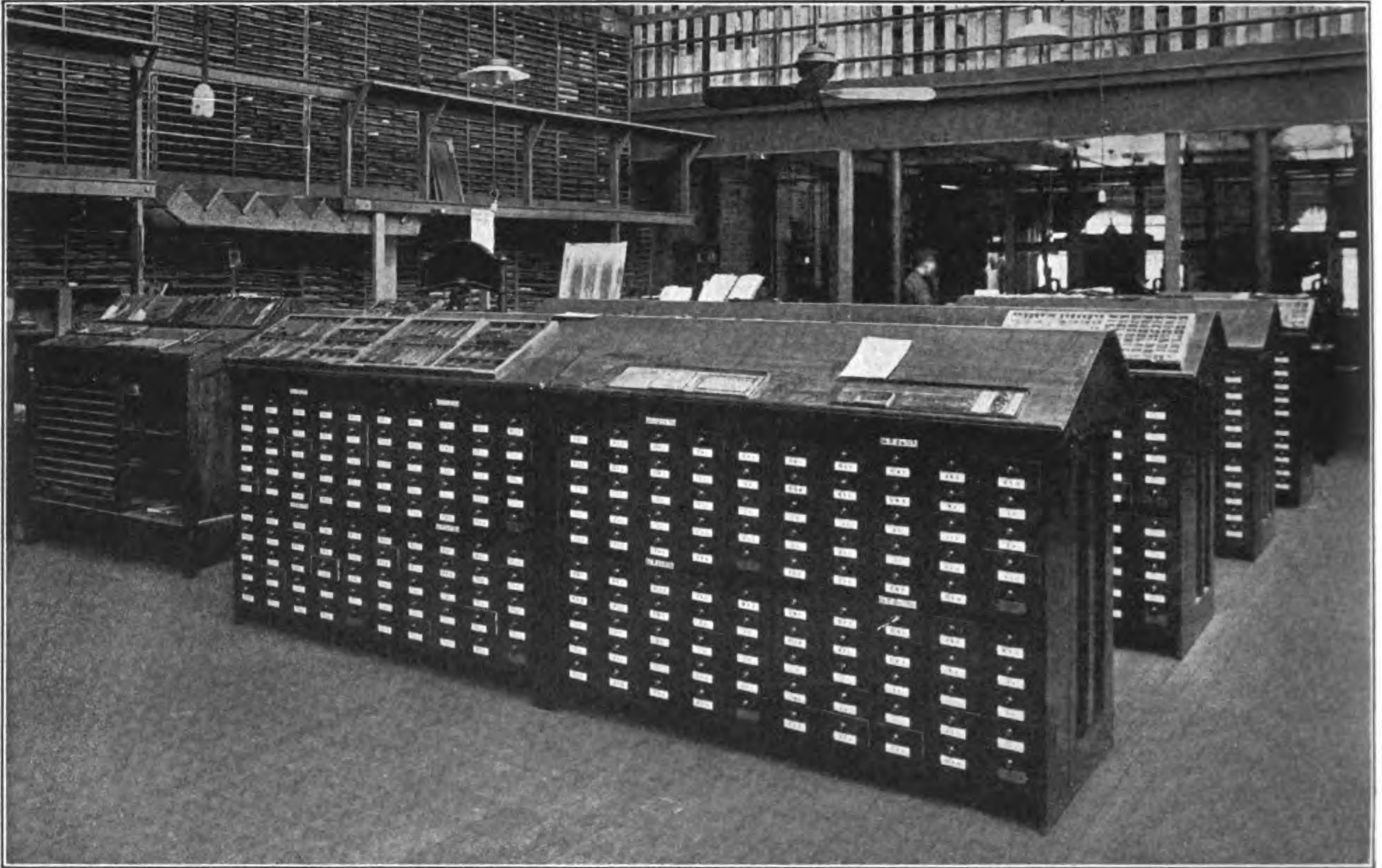
The "Book Side" at the Hugh Stephens Plant, Jefferson City, Mo., showing arrangement of sort cabinets. Each alley contains a complete assortment of Monotype faces. Men do not leave alley at any time. Eight complete plants in one
