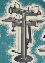
Router, Jigsaw and Type High
