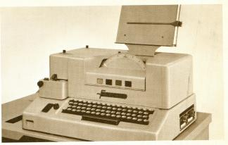
UNIVERSAL PERFORATOR — Permits mixing of type faces regardless of quad size and/or lower case alphabet length. Interchangeable magazines make the Universal Perforator capable of setting a virtually unlimited combination of type faces up to 18 point.
