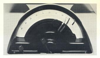
Large counting scale is stationary, and finished in non-glare white enamel. Justification range is easily located by the operator since the area justification remains in fixed position. The operator can set the indicator pointer to the column measure... without having to refer to a chart.
