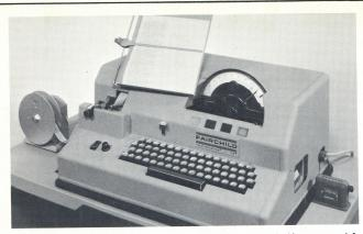
MULTIFACE PERFORATOR — Designed primarily for use with conventional (non-unit) matrices. Serves many newspapers as well as commercial shops. Has added flexibility of interchangeable counting magazines which accommodate any font from 5 to 14 point.
