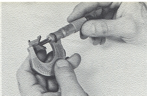
Operator "mikes" matrix preparatory to selecting matching code blade for insertion in counting magazine.
