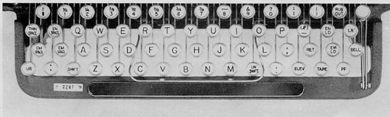
FIGURE 16. Teletypesetter Standard Perforator keyboard layout when fractions are required.
