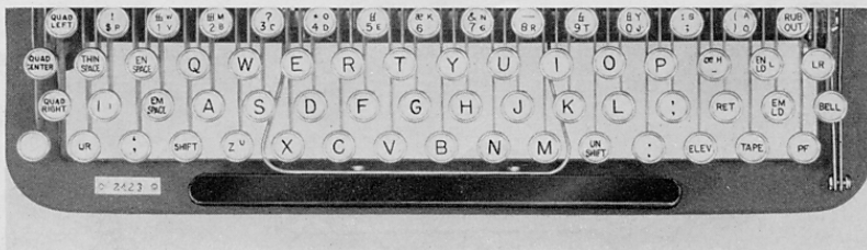
FIGURE 18. Teletypesetter Multiface Perforator keyboard layout when small caps are required.
