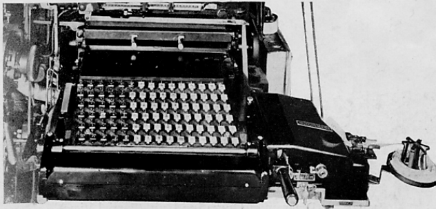
FIGURE 11. Teletypesetter Operating Unit Attached to Linecasting Machine.
