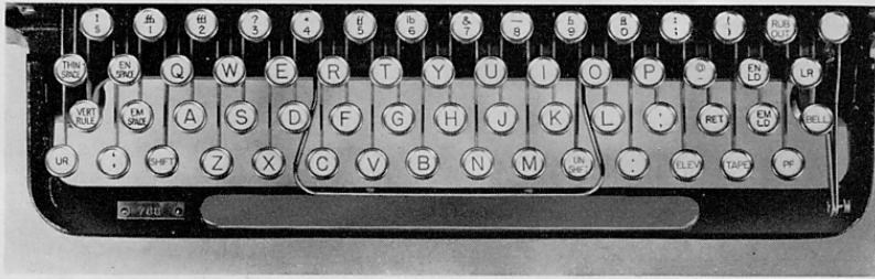
FIGURE 15. Teletypesetter Standard Perforator keyboard layout when fractions are not required.
