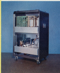
The console cabinet is on rollers, and may be placed in any convenient position. If necessary it may be rolled behind the machine to save floor space. Pull drawers contain all circuitry, and when extended, make routine examination easy for the maintenance men.
