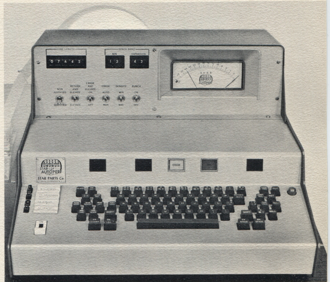
Operation of the AutoPerf is easy to learn. Its built-in "intelligence" makes most line-ending decisions and automatically prevents tight or loose lines from elevating.
