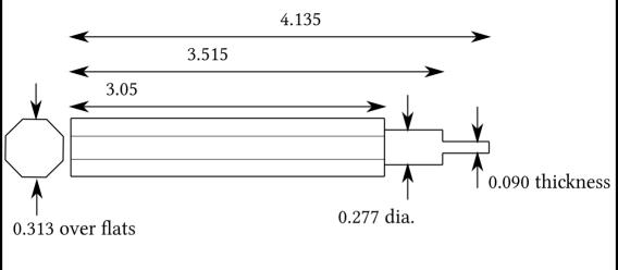
Punch'D' ("Ear Punch"), probably shop-made replacement, for Star Matrix Repair Tool.
