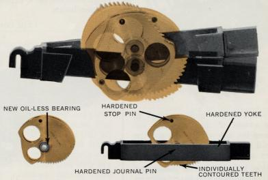
The new Star oil-less keyboard cams never require lubrication. They are equipped with engineered plastic bearings, which revolve on hardened journal pins. These special bushings practically eliminate friction and reduce maintenance to near zero.
