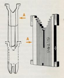
A. Edge of spaceband and quad matrix (mold height plane)
