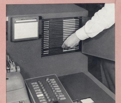
Linofilm font grids consist of 88 negative characters on a sturdy glass plate, and are housed in this turret. Font grids automatically swing into operating position as called for.
