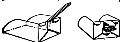
A Small Square Scoop Made of Tin for Dipping Up Shot Stored in a Square Bin
